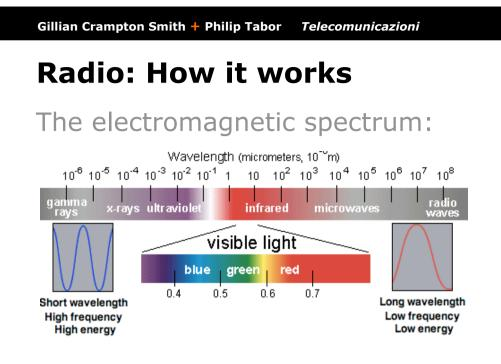
Electromagnetic energy is radiated as waves.
