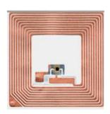
An RFID tag is a chip and a 'transponder' (radio transmitter-responder).
