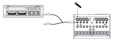
2. Bypassing the IO | 14/26's preamplifier – The IO | 14/26 has excellent sounding preamplifiers built in, but if you have a megabucks or vintage preamp that you want to use instead, experiment with connecting it to the insert jack. The insert jack allows you to use your external preamp while completely bypassing the IO | 14/26's built in preamplifier.
