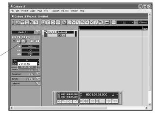
If you want to monitor your audio with Cubase's effects (distortion, reverb, etc.), press the direct monitoring button next to the Record Enable button.
