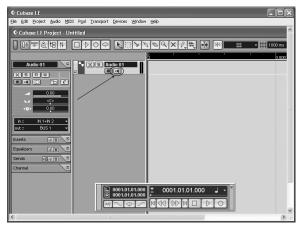
Using Cubase's direct monitoring requires the audio to make a round-trip through the computer, which causes a small but noticeable delay as the digital audio is processed. To avoid any echo effects, open the Alesis Hardware Direct Monitoring panel and mute the corresponding input. This way, you will only hear the signal with effects without also hearing the pure signal output from the IO.
