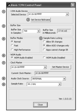
To open the control panel from within Cubase in Windows, select "Devices" | "Device Setup...." | "VST MultiTrack." Then, click the "Control Panel" button.
