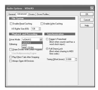
A limitation of the WDM architecture is that, each time you change between "low" (44.1/48), "medium" (88/2/96), and "high" (176.4/192) sample rates, the WDM profiler needs to be run again.
